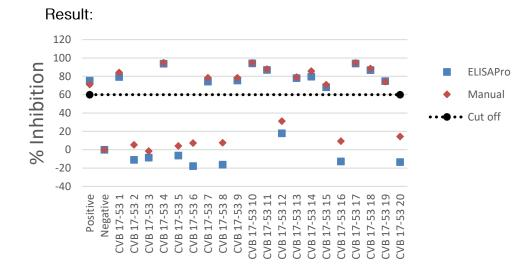
Cross-contamination Confirms there is no well to well cross-contamination due to carryover of samples
