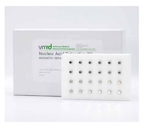
The magnetic separator is designed for use with the magnetic bead extraction kits in either the U-bottom or square well block plates. To separate the beads from the solution, the separation plate is seated/placed onto the magnetic separator. The beads are attracted to the magnet and collect against the walls of the plate wells (or tube), allowing for removal of wash buffers and/or recovery of elution liquid.
